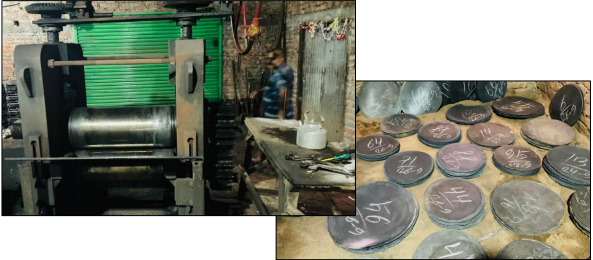
Fig.3 & 4. Snapshot of the rolling mill and the bell metal plates for processing
